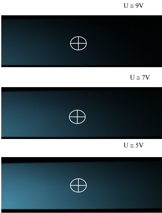
Figure 4: Observed optical angular effect observed with a camera with the objective focused in the center of the LCD
