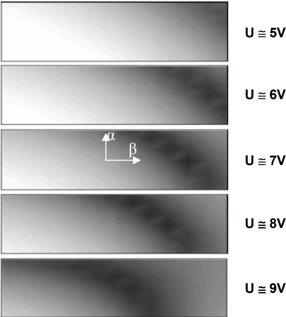
Figure 7: Simulated light transmission of the TN LCD, where \alpha and \beta are the angles of the optical angular effect
