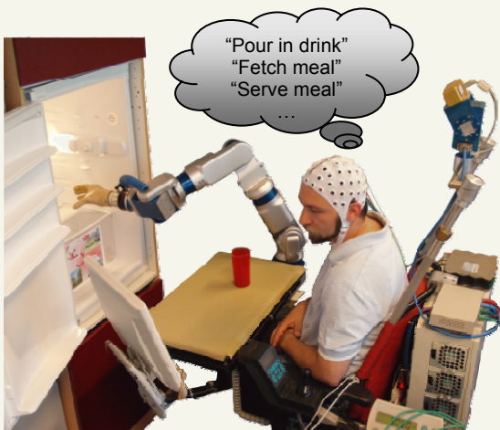
Figure 1: Commanding a service robot on high abstraction level (here with brain computer interface)
